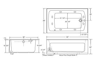
Skirted baths can be ordered as above floor rough models with factory-installed 2-1/4" risers if required.
