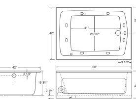
Skirted baths can be ordered as above floor rough models with factory-installed 2-1/4" risers if required.
