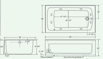
NOTE: All dimensions and specifications are nominal and may vary  $\pm 1/4$ ". Use actual products for accuracy in critical situations. All whirlpools require a single 115V/20 amp GFCI circuit.
